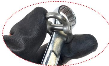
**4** Assure that the tool will not pass the pin by sliding/twisting it until it stops, then slide/twist it the opposite direction and again assuring it stops. For the best functionality and use, choose the side of the Double Dee that provides the most freedom but still contained.
