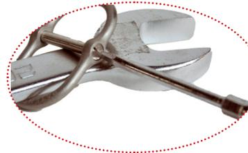
**5** Once it is threaded properly, tighten the pin by using a straight or flat end screw driver. While installing the pin, resistance will be felt as the c-clip starts to enter the hidden groove in the bore.
