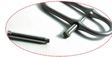
**6** To assure the pin is engaged properly, try to back out the pin using very light pressure- if there is resistance felt the pin is engaged properly, if not remove the pin and install a new one.
