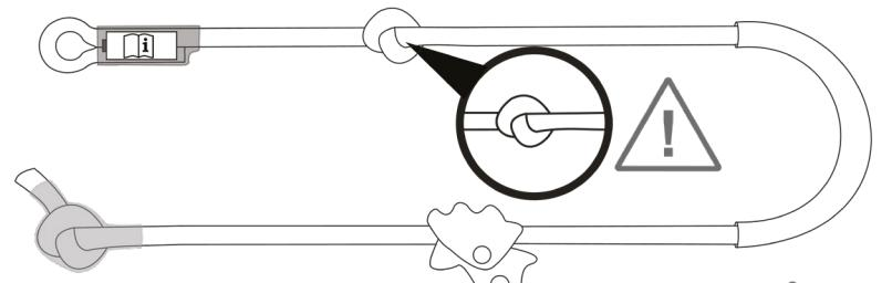
If used according to EN 795, length adjustment not permitted.
