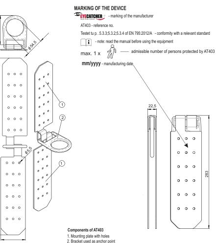
TIME OF USAGE - The anchor point can be used for 5 years from the date of the first use. Following the first five years of usage the manufacturer's inspection must be carried out.
