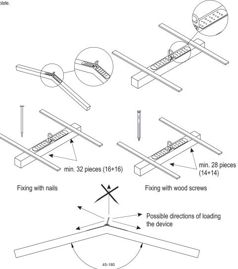
The device AT 403 can be installed only on wooden beams with dimensions of no less than 70x70 mm.
