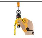
The rope can be installed with the device connected to the anchor.
