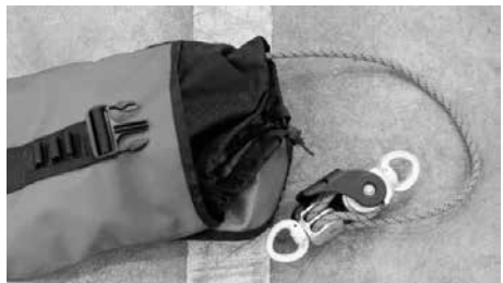
Pulleys secured for storage
