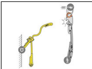
If the helicopter needs to suddenly leave its stationary position, the adjustable arm ejects instantly to free the victim, rescuer and helicopter.
