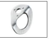
Petzl hangers are textured on the back side that is in contact with the structure (concrete, rock, or other). This helps prevent the hanger from turning when the anchor is being installed or when it is heavily laterally loaded during use.
