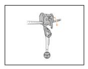
The ergonomic captive carabiner allows the guide to quickly install the trolley on the cable with one hand.
